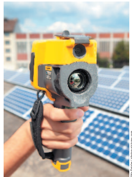
▲ So many choices: Some users prefer cameras with pistol grips (here, the Fluke TiR32), while others swear by cameras with a rotatable display.
